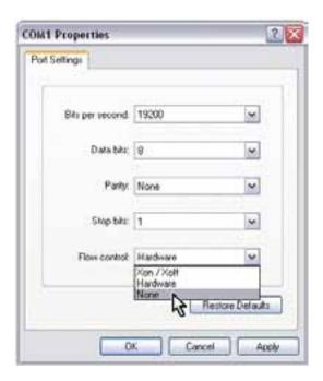
Click OK, normally Hyperterminal will connect automatically, you are ready to start the communication between PC and PM1122 interface.
