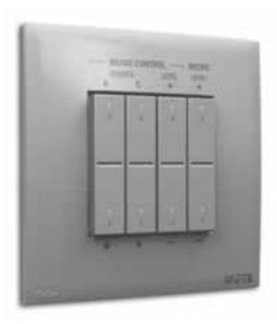
4 buttons named A to D are used for selecting the source or to recall a preset. By default, these buttons are used to select source A to D. Next to that are an up and down button controlling the music level and finally the same 2 buttons controlling the microphone level.
